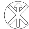
Signal device LED arrow-cross (installed in the housing or in the cover plate on both sides).
